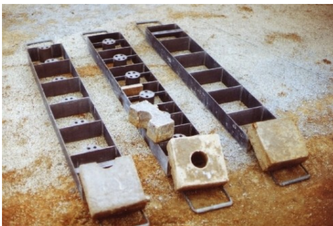
Photo taken of our three steel molds which cast different shaped bricks for our construction purposes.
